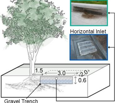
Measurements were made of stormwater runoff captured in trenches via: 1) vertical or 2) horizontal inlets.
